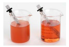
Fluid volume: 250 gallons, 1000 liters Initial ppm H<sub>2</sub>O: 12000 ppm, Final ppm H<sub>2</sub>O: < 50 ppm
