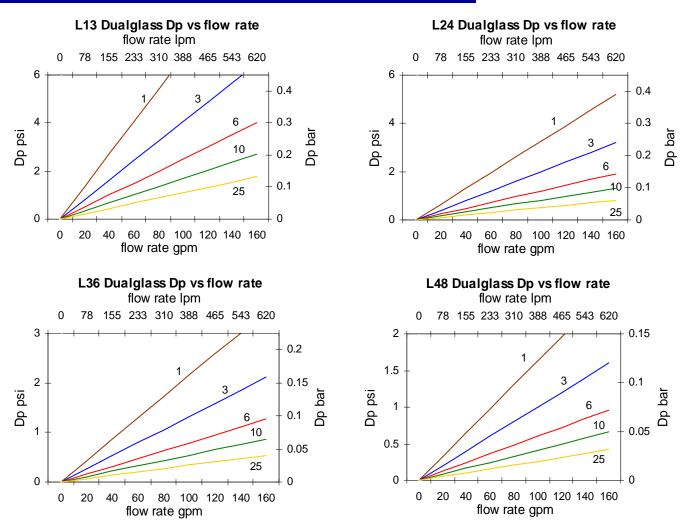
Pressure drop curves based on oil viscosity of 150 SSU, and specific gravity = 0.9. Dp across element is proportionally related to viscosity and specific gravity. For new DP use the following conversion formula: DP element = DP curve x Actual Viscosity/150 x Actual SG/0.86
